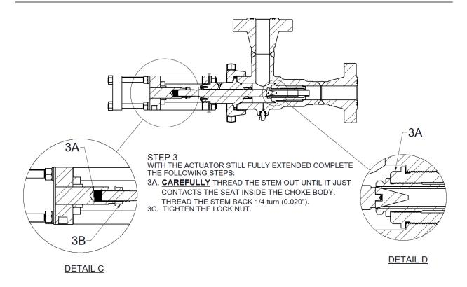
Adjusting the stem back away from the seat will avoid the risk of damage as the choke stem should not contact the seat when fully extended. ¼ turn (0.020") is equivalent to approximately 13/64, this must be considered when calibrating any position sensors.
