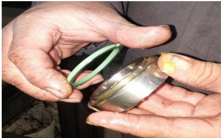
5. Apply a moderate amount of **grease** onto the bottom seal pocket of the **BV Body (#9)** then install the first **Seat Carrier Assembly**.
