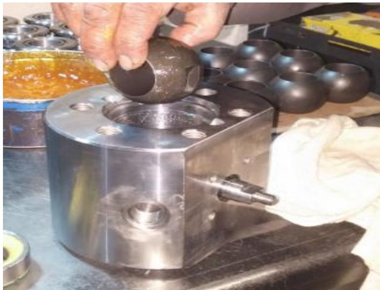
10. Install the second **Seat Carrier Assembly** on top of the **BV Ball** with the **L-Seal** facing up.
