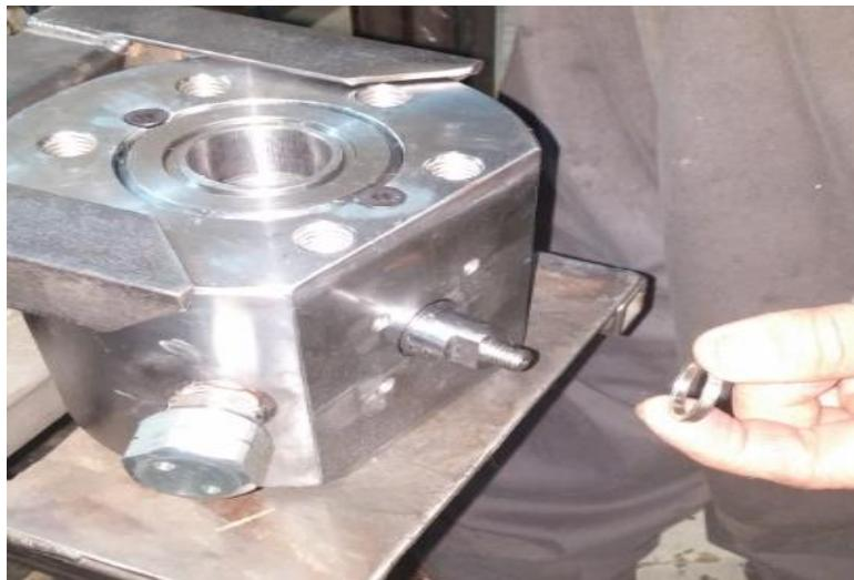
**18.** Slide the **Belleville Washer (#12)** onto the **BV Stem** next to the **BV Packing Ring**.
