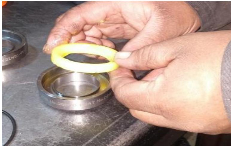
3. Install the **BV Seats** into the seal pocket of the **Seat Carriers** by tapping them with a rubber mallet until fully engaged.
