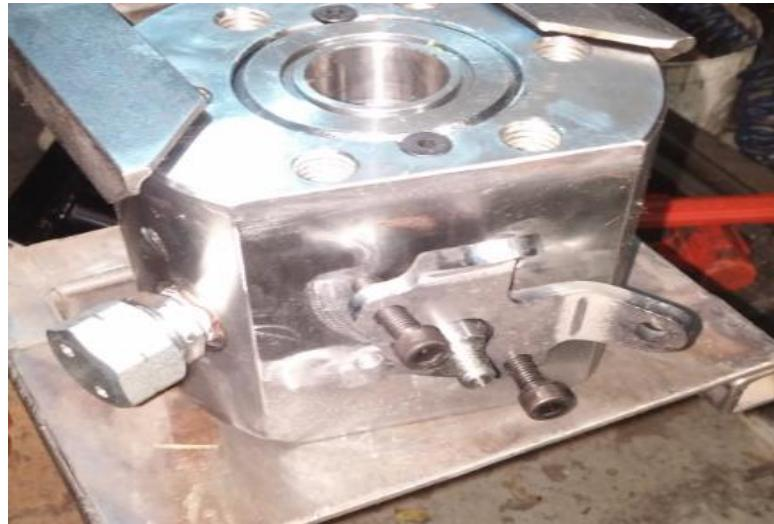
**20.** Attach the **BV Handle (#15)** onto the **Stem** as shown then secure it with the **Hex Flange Nut (#16)**.
