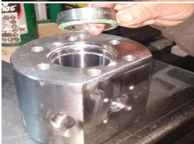
6. Apply a moderate amount of **grease** on the **BV Stem (# 20)** and the **BV Stem Washer (#19)**. Slide the **Stem Washer** onto the **Stem** up against the shoulder.
