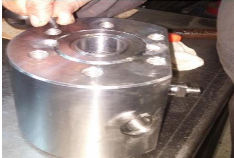
**14.** Coat **O-Rings (#2)** with **grease** then install them into the external groove of the **Seat Retainer** and on the other end of the **BV Body**.
