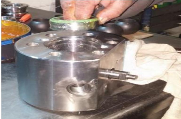
11. Coat **O-Ring 144 (#4)** with **grease** then install it into the groove of the **Seat Retainer (#3)**.
