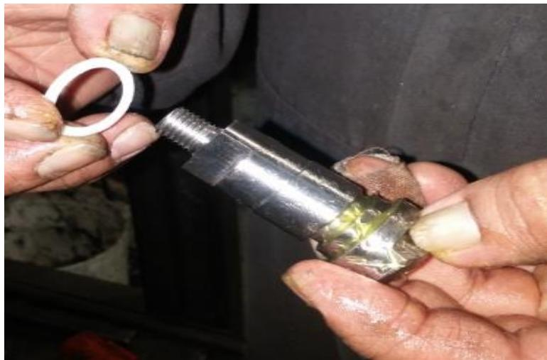
7. Coat O-Ring 114 (#18) with **grease** then slide into the groove on the **BV Stem**.
