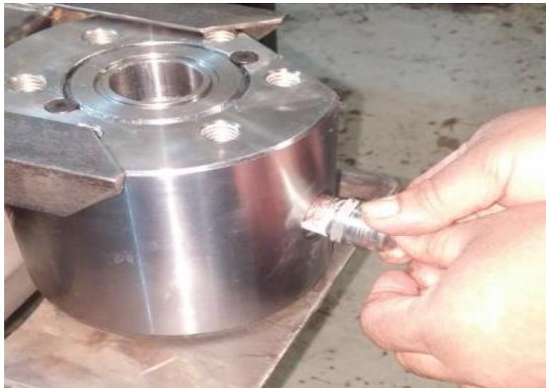
**16.** Slide the **BV Stem Packing (#10)** onto the **BV Stem** up into the seal pocket on the **BV Body**.
