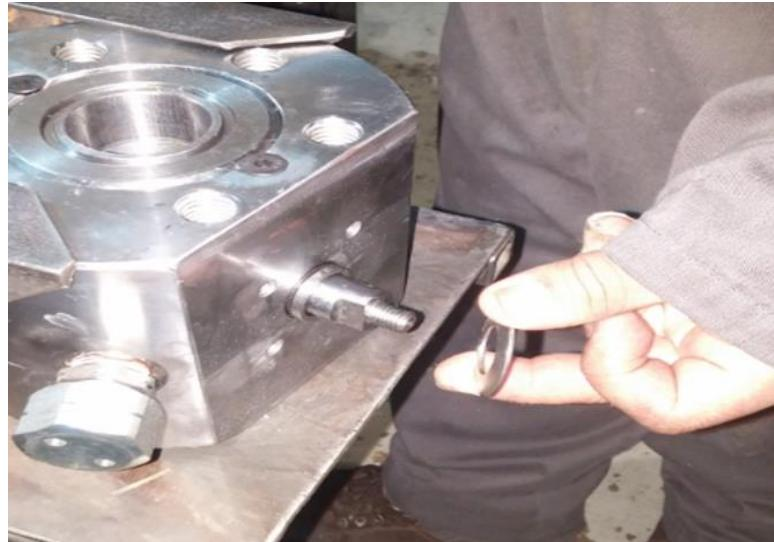
**19.** Slide the **BV Gland Plate (#13)** onto the **BV Stem** up to the **Belleville Washer** with the orientation as shown. Apply **anti-seize compound** on the threads of the **Cap Screws (#14)** and insert them through the **BV Gland Plate** into the threaded holes on the **BV Body** and tighten until the **BV Gland Plate** is below the shoulder of the **BV Stem**.
