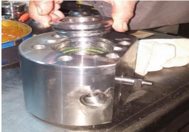
**13.** Apply **anti-seize compound** on the threads of the **Countersunk Screws (#1)** then thread them into the end of the **BV Body** and tighten them snugly.
