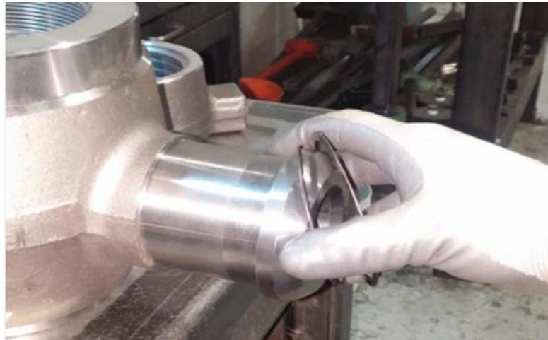
3. Slide the **Wingnut (#18-2)** next to the **Snap Ring**. Place the **Segment Set (3) (#18.3)** around the male end and pull the **Wingnut** over the **Segments** to hold them in place.
