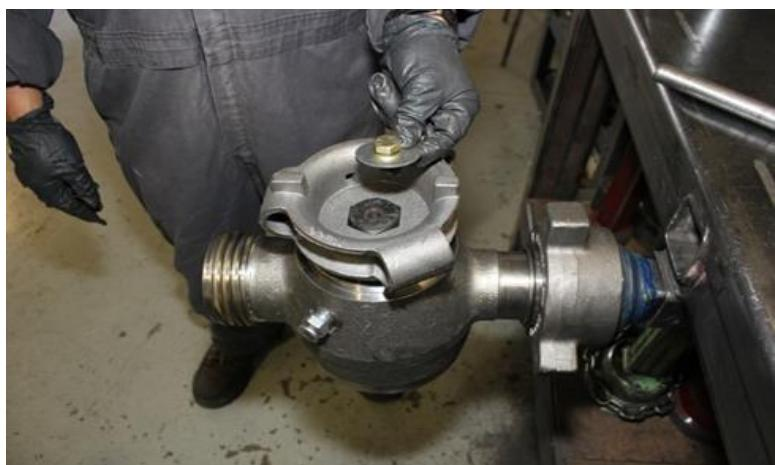
**22.** **Grease** the **Plug Valve** with **RDI-2015 performance grease** before and after hydro test.
