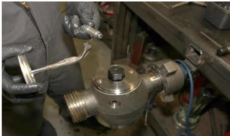
18. Apply an **anti-seize compound** on the threads of the **Socket Head Cap Screw (#6)** then thread it into the hole (male end side) of the **Plug Valve Body** as shown.
