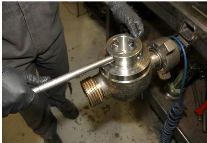
17. Apply an **anti-seize compound** on the threads of the **Safety Tap Fitting (#17)** and screw it **clockwise** into the side threaded port on the **Plug Valve Body**. Torque the **Safety Tap Fitting** to 80 ft. lbs.
