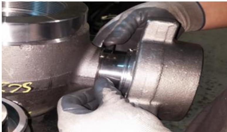
5. Insert the **Union Seal (#9)** into the inside groove at the female end of the **Plug Valve Body**.
