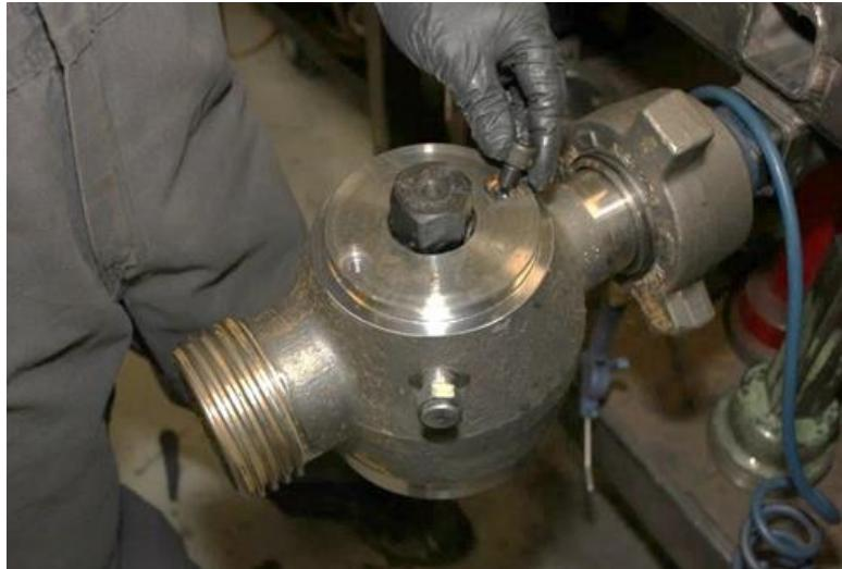
19. Slide the **Stop Plate (#5)** onto the **Plug Body** hex as shown for proper orientation - **open position**.
