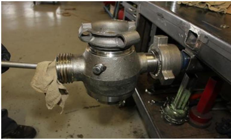
24. Complete a final inspection to ensure that the bores of the **Plug**, **Seats** and **Valve Body** are aligned in the open position. Adjustment can be done by threading the **Cap** in or out of the **Body** as required.
