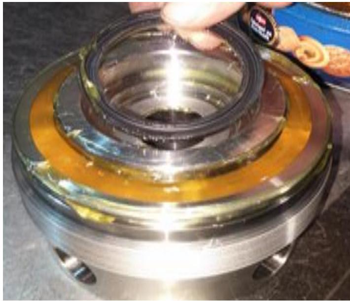
9. Lightly **grease** **O-Ring (#14)** and install into the outer groove of the **Cap Body**.
