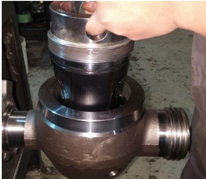
16. Using a bar, tighten the **Cap Body** until snug, then back off a  $\frac{1}{4}$  turn to allow free movement of the **Plug Body**.
