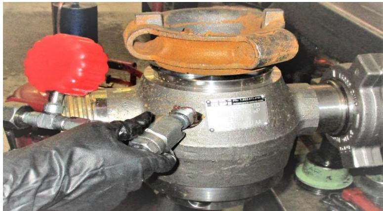
23. Remove the excess **grease** in the bore of the **Plug Valve** by pushing a clean rag through the bore.
