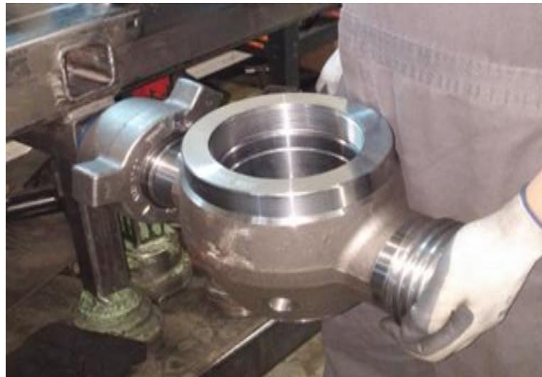
6. Insert and punch the **Grooved Pins (#7)** into the internal pin holes on both sides of the **Plug Valve Body**.
