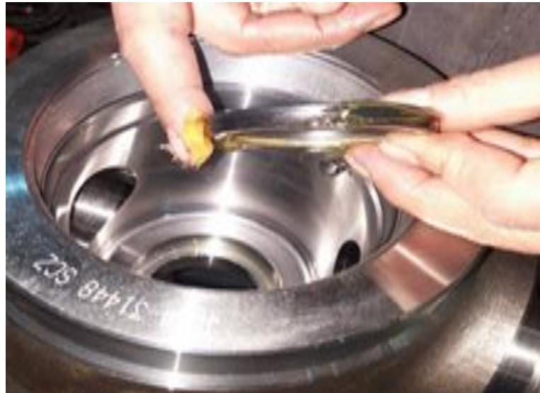
8. Pack the **Cap Body (#15)** with **grease** all around the open groove as shown. Apply **grease** into the seal pocket of the **Cap Body** and on **Plug Seal (#10)**. Insert the **Plug Seal** into the **Cap Body** seal pocket - **copper plate facing down**.
