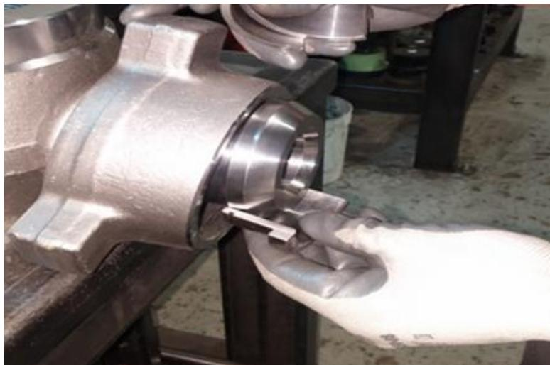
4. Pry the **Snap Ring** around into the machined groove on the **Segments** to secure the **Wingnut Kit** together.
