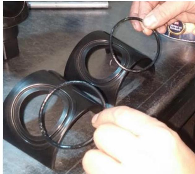
**13. Clip the **Seat Carriers** around the **Plug Body** - anchoring them on the groove of the **Cap Body** as shown.**
