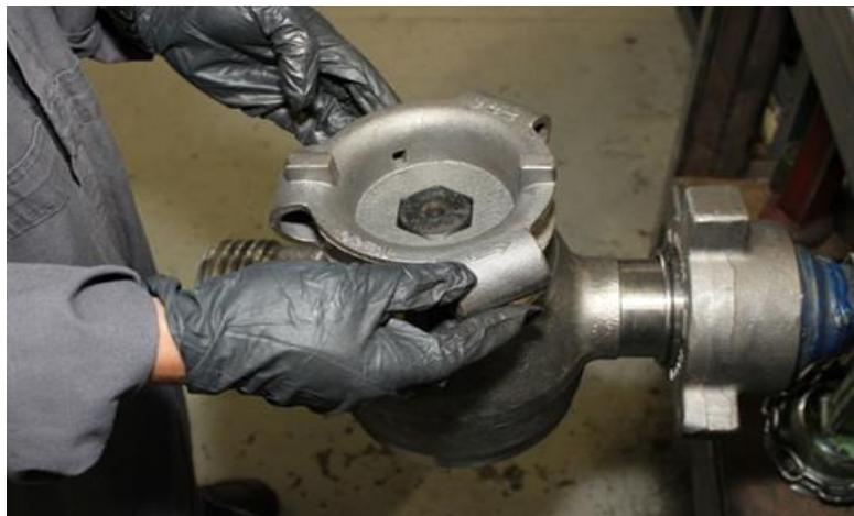
**21.** Secure the **Handle** with the **Hex Bolt (#1)** and **Washers (#2 & #3)** - tighten till snug. Recheck the **1/2 Hex Bolt** on the other end of the **Plug** - **tighten if necessary**.
