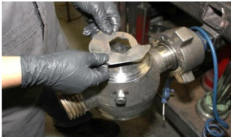
**20.** Place the **Plug Valve Handle (#4)** over the **Stop Plate** with indicator tabs aligned to the **Plug Valve Body**.
