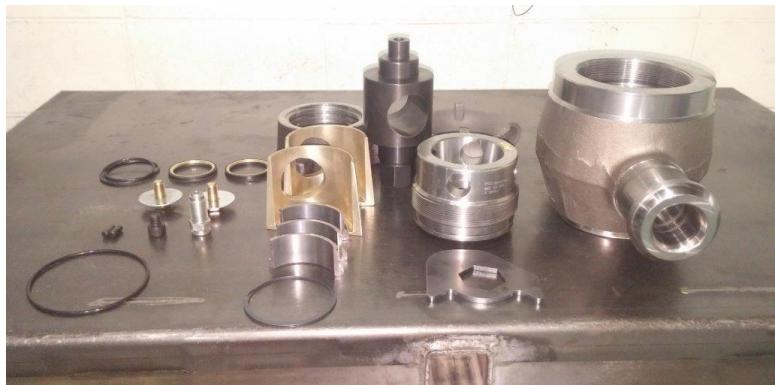
2. Install the **Snap Ring (#18-1)** onto the male end of the **Plug Valve Body (#8)**.
