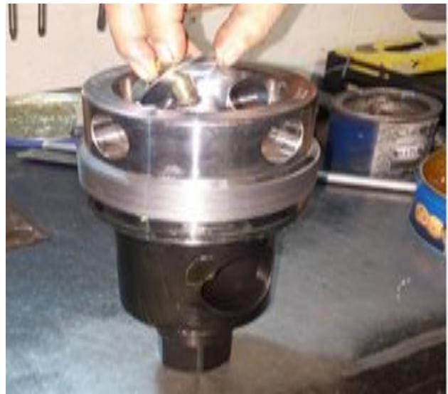
**12. Apply **grease** on **O-Rings (#13)** and install into the groove of the **Seat Carriers (#12)**. Then apply **grease** on the sealing area of the **Seat Carriers - concave side**.**
