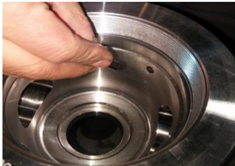
7. Apply a moderate amount of **assembly grease** to the **Plug Valve Body** seal pocket (the very bottom of the **Plug Valve Body**) and on the **Plug Seal (#10)**. Insert the **Plug Seal** into the **Plug Valve Body** seal pocket - copper plate facing down.
