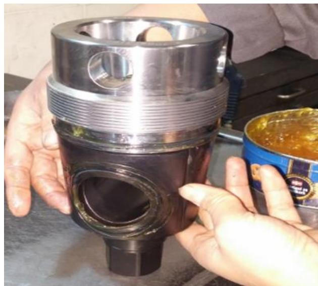
14. Apply an **anti-seize compound** on the external threads of the **Cap Body** and onto the corresponding threads of the **Plug Valve Body**.
