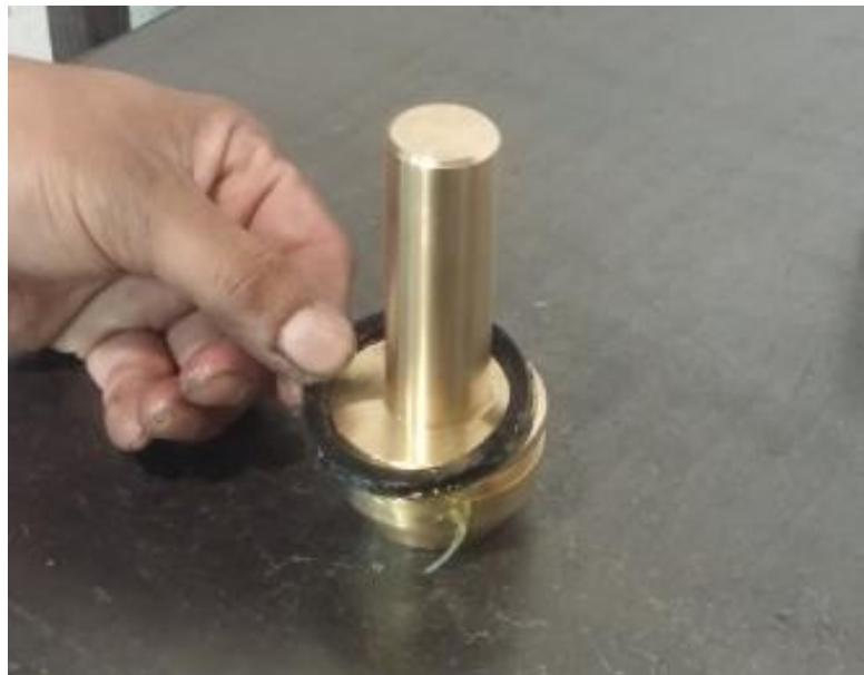
**10.** Apply [anti-seize compound](#) on the internal threads of the **PRV Body**.
