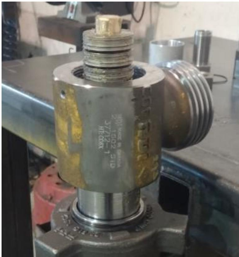
**13.** Coat O-Ring 038 (#8) with **grease** and install it into the groove of the **Cap (#7)**.
