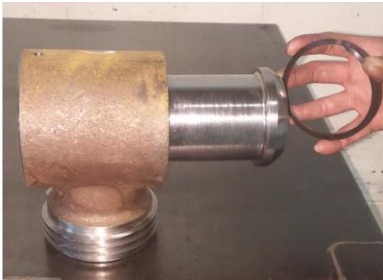
**3. Slide the Wingnut Body (#19.2) onto the male end up against the PRV Body and Spiral Retaining Ring. Place the Segment Set (3) (#19.3) around the male end and pull the Wingnut Body over the Segments to hold them in place.**
