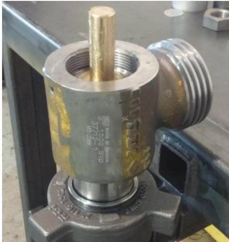
**12.** Apply a liberal amount of **grease** on the **Disk Springs (16 pcs) (#9)** and slide them onto the **Keeper** with the first two concave springs facing up then two concave springs facing down - repeat the sequence for the rest of the springs.
