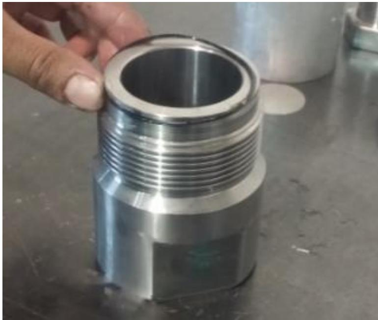
**14.** Apply **anti-seize compound** on the threads of the **Cap** then thread it into the **PRV Body** and tighten snugly.
