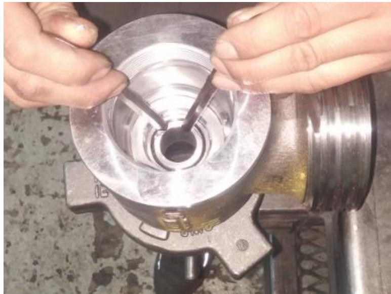
6. Coat the **Seat (#14)** with **grease** and place on top of the **O-Ring 028** with bevel side facing up.
