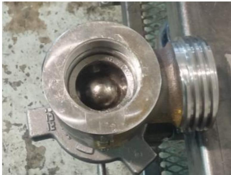
9. Coat the **Loaded U-Cup (#11)** with **grease** then install into the groove of the **Keeper (#10)** with concave side facing down.
