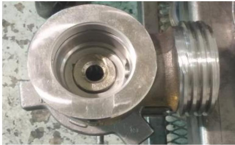
7. Coat the **Spider (#13)** with **grease** and place on top of the **Seat**.
