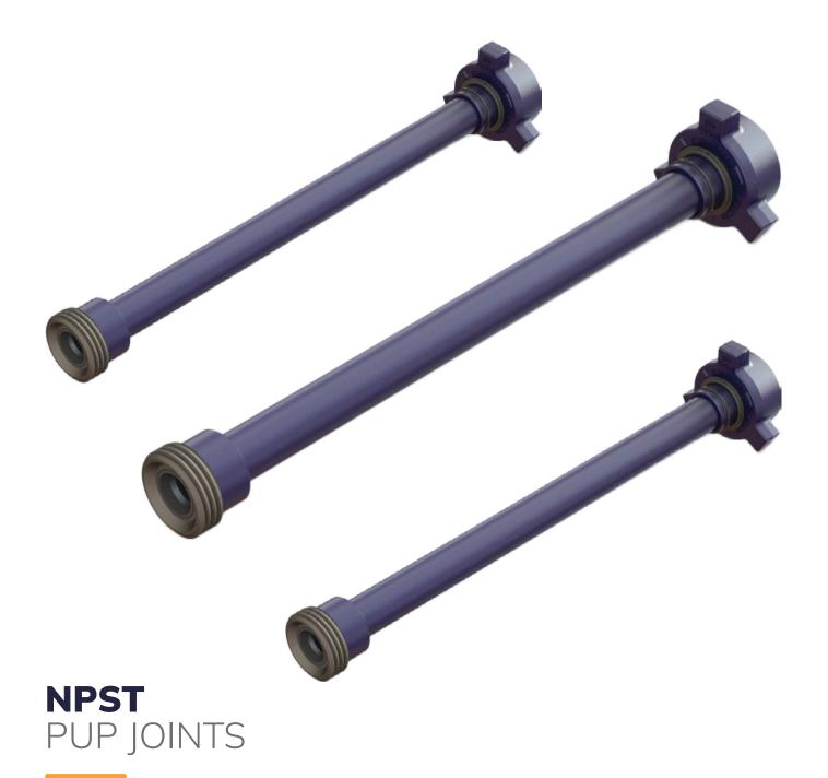
**RDI's Non-Pressure Seal Thread (NPST) Pup Joints** are a lightweight pup capable of up to 15,000 psi NSCWP. The NPST pup joints are available with an optional detachable wing nut that allows fast, easy on-site serviceability. RDI's NPST pup joints are well suited for abrasive applications where a smooth bore is needed to assure minimum turbulence.
