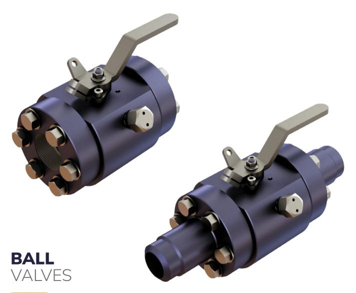
RDI's Ball Valves are designed as an economical light-weight alternative to plug valves, while still maintaining an integral design. The floating ball design assures bubble-tight sealing at pressure, and the standard grease fittings allow the user to flush abrasives from the sealing face. The RDI ball valve is available in pressures up to 10,000 psi NSCWP†.
