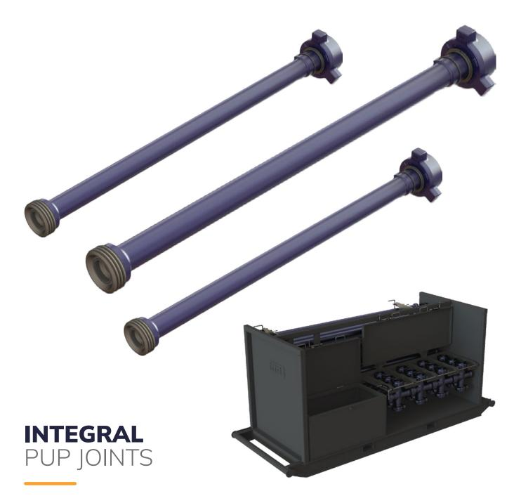
**RDI's Integral Pup Joints** are designed and manufactured from seamless, forged one-piece construction to give a smooth uninterrupted bore and greater flow. They are used on high pressure discharge lines, flowlines and choke and kill lines. RDI Integral Pup Joints are available in pressures up to 15,000 psi NSCWP<sup>†</sup>.
