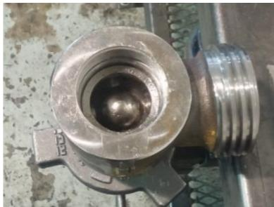
9. Coat the Loaded U-Cup (#11) with grease then install into the groove of the Keeper (#10) with concave side facing down.
