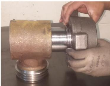
Mount the **PRV Body** on a bench receiver.
