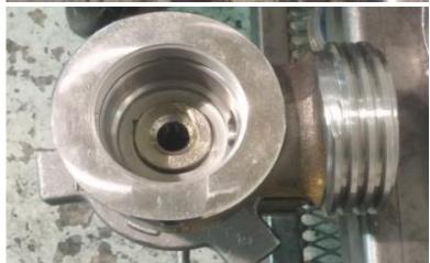
Coat the Spider (#13) with grease and place on top of the Seat.
