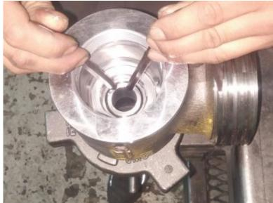
Coat the Seat (#14) with grease and place on top of the O-Ring 028 with bevel side facing up.
