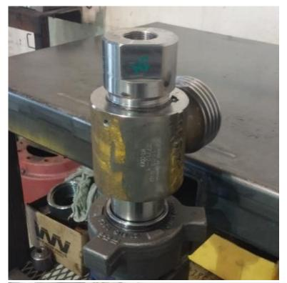
15. Apply anti-seize compound on the threads of the Adjusting Screw (#5) then thread the Hex Nut (#6) all the way onto the Adjusting Screw. Install the Adjusting Screw into the Cap until it just touches the Keeper.
