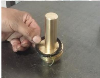
Apply anti-seize compound on the internal threads of the PRV Body.
