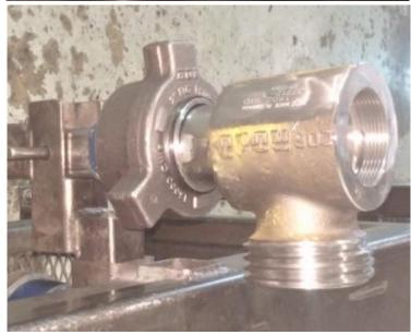
5. Coat O-Ring 028 (#15) with grease then install into the groove in the PRV Body.
