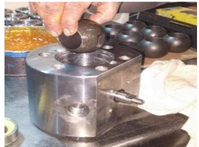
10. Install the second Seat CarrierAssembly on top of the BVBall with the L-Seal facing up.
