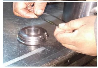
**12.** Apply a moderate amount of **grease** onto the upper groove of the **BV Body** then install the **Seat Retainer Assembly**.
