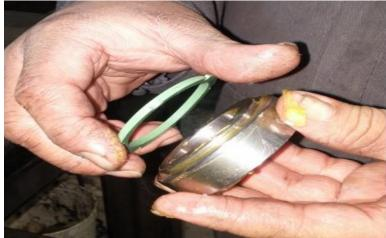
5. Apply a moderate amount of grease onto the bottom seal pocket of the BV Body (#9) then install the first Seat Carrier Assembly.
