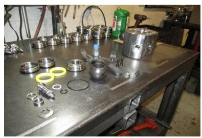
2. Apply a moderate amount of grease onto the seal pocket of the Seat Carriers (#6) and the Ball Valve (BV) Seats (#7).
