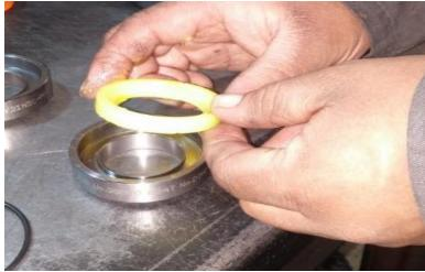
Install the BV Seats into the seal pocket of the Seat Carriers by tapping them with a rubber mallet until fully engaged.
