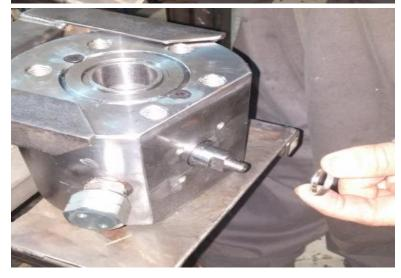
**18.** Slide the **Belleville Washer** (#12) onto the **BV Stem** next to the **BV Packing Ring.**
