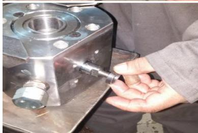
17. Slide the BV Packing Ring (#11) onto the BV Stem next to the BV Stem Packing.
