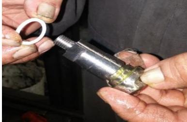
7. Coat O-Ring 114 (#18) with grease then slide into the groove on the BV Stem.
