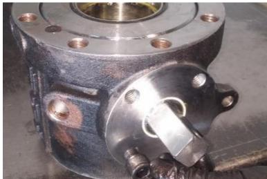
**14.** Slide the **Stop Plate (#16)** onto the **Stem** in the position and orientation as shown.
