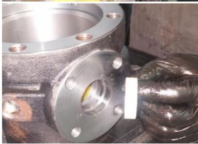
Insert the Stem Assembly into the "stem hole" of the BV Body until fully engaged.
