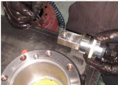
Coat Stem Washer (#15) with grease then install it into the external pocket groove of the BV Body.
