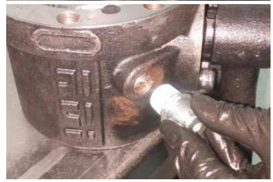
**18.** Replace the Venting Cap of the **Body Grease Fitting**.
