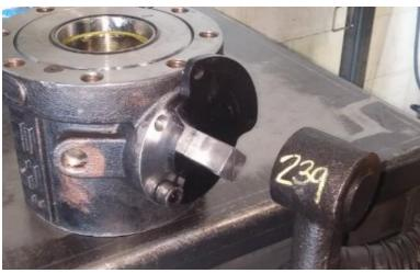
17. Remove the Venting Cap of the Body Grease Fitting (#13) and apply 3-4 turns of Teflon tape on its 1/2 NPT threads. Thread the Body Grease Fitting into the side threaded hole of the BV Body and tighten it snugly.
