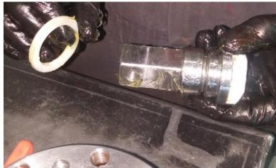
Coat O-Ring 216 (#12) with grease then slide it onto the Stem into the groove.
