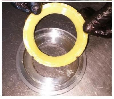
9. Coat O-Ring 247 (#4) with grease then install it into the groove on the Seat Retainer.
