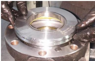
11. Apply anti-seize compound on the threads of the Countersunk Screws (#1) then thread them evenly into the BV Body to secure the Seat Retainer.
