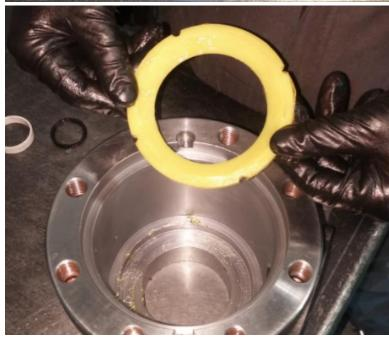
3. Apply a liberal amount of grease on the Stem (#10) and Thrust Washer (#11). Slide the Thrust Washer onto the Stem up against the shoulder.
