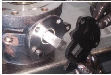
15. Attach the Handle (#17) with the Handle Cap (#19) onto the Stem as shown.
