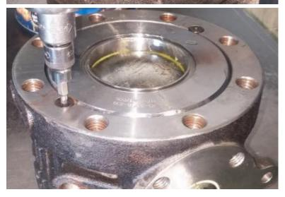
12. Coat the two O-Rings 235 (#2) with grease then install them into the external groove of the Seat Retainer and into the bottom groove of the BV Body.
