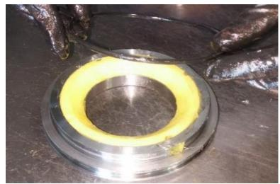
10. Apply a moderate amount of grease into the upper groove of the BV Body then install the Seat Retainer Assembly.
