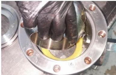
8. Apply a liberal amount of grease on the seal pocket of the Seat Retainer (#3). Coat the second Seat with grease then install it into the seal pocket of the Seat Retainer.
