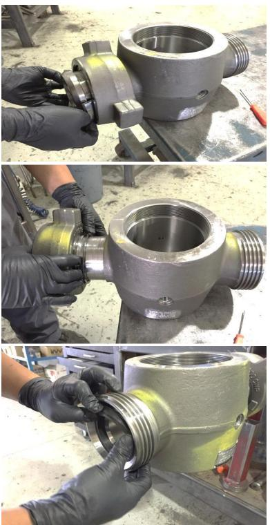
Mount the **Plug Valve Body** on a bench receiver.
