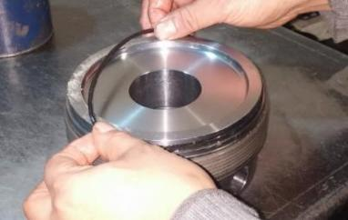
17. Grease the sealing surface of the Cap Body. Apply anti-seize compound on the threads of the Cap Body and the corresponding threads of the PV Body.
