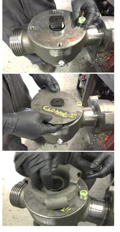
23. Grease the Plug Valve with RDI 2015 performance grease before and after Hydro Test.
