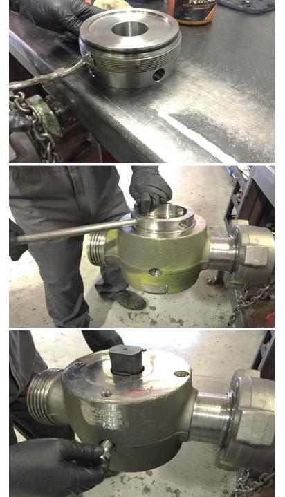
19. Turn the PV Body upside down. Apply anti-seize compound on the threads of the two (2) Button Grease Fittings (#5) then thread them into the sides of the PV Body and tighten them snugly. 20. Apply anti-seize compound on the threads of the Socket Head Cap Screw (#3) then thread it into the top of the PV Body on the male side and tighten it snugly.
