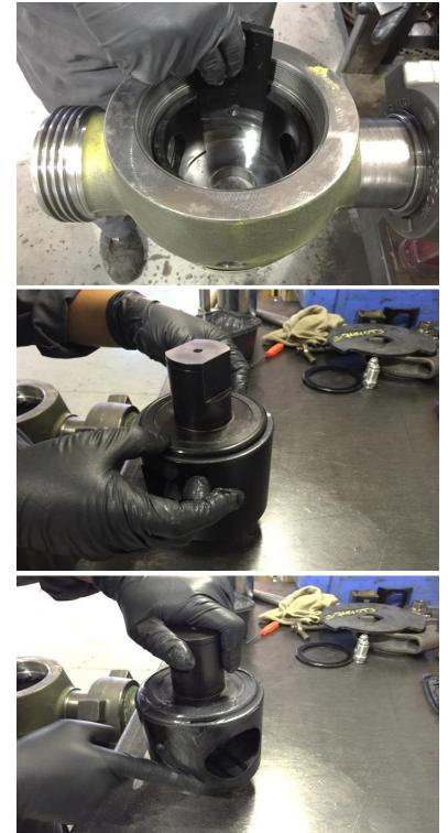
13. Apply a liberal amount of assembly grease on the Plug Body including the Plug Seal that was just installed.
