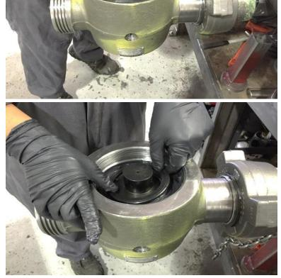
Coat the second Plug Seal with grease then install on the Plug Body.
