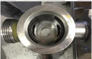
11. Grease both sides of the Seat Carrier Spacers (#11) then insert them between the Seat Carriers flush to the wall of the PV Body.
