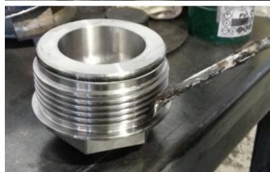
**13.** Install the **Cap** to the **SCV Body**. Tighten **clockwise** until snug.
