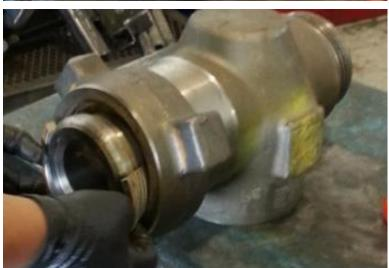
Pry the Spiral Snap-Ring around into the groove of the Segments to secure the Wingnut.
