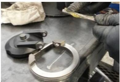
7. Align the pin holes of the Clapper and Clapper Hanger then insert the Dowel Pin as shown.
