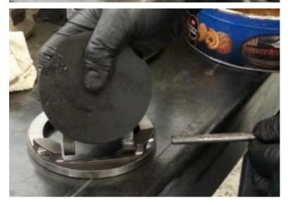
8. Grease the corresponding sealing surface of the Clapper inside the SCV Body.
