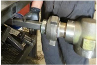
Grease Dowel Pin (#6) and the pin holes of the Coated Clapper (#4) and Clapper Hanger (#5).
