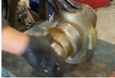
4 Slide the Wingnut (#3.2) onto the male end up to the Spiral Snap Ring. Place the Segments Set (3) (#3.3) around the male end and pull the Wingnut over the Segments to hold them in place.
