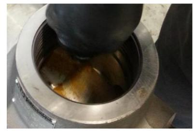
9. Place the Hanger-Clapper Assembly into the SCV Body flat sealing surface of the Clapper against the flat sealing surface inside the SCV Body.
