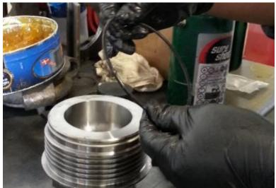
**12.** Apply anti-seize compound on the threads of the Cap and to the corresponding threads of the SCV Body.
