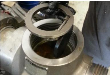
10. Ensure that the Hanger-Clapper Assembly sits evenly on the internal ledge of the SCV Body.
