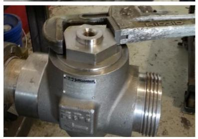
**14.** Apply anti-seize compound on the threads of the **Eyebolt (#9)**. Install and tighten the **Eyebolt** until snug.
