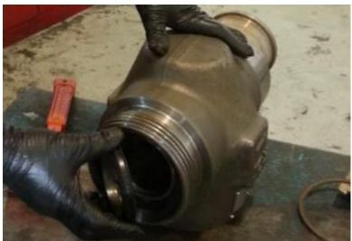
3. Install the Spiral Snap-Ring (#3.1) onto the male end of the SCV Body.
