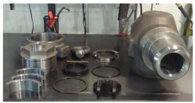
2. Install the Union Seal (#1) into the groove in the female end of the Swing Check Valve (SCV) Body (#2).
