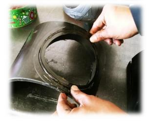
8. Install the Seat Carriers onto the Plug Body.
