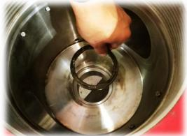
**15.** Apply anti-seize compound on the internal threads of the **Plug Valve.**
