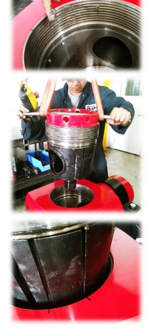
17. Using a bar, tighten the Cap Body till snug, then back off a ¼ turn to allow free movement of the Plug Body.
