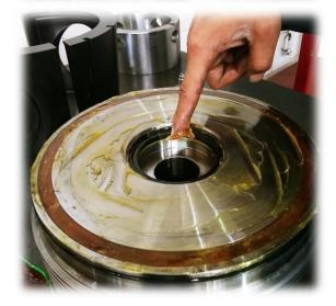
Apply a liberal amount of RDI 2015 (grease stick) on the sealing surface of the Plug Body (#11).
