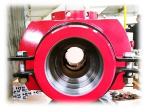
19. Thread the two remaining Giant Button Head Grease Fittings into both sides of the Plug Valve - tighten till snug.
