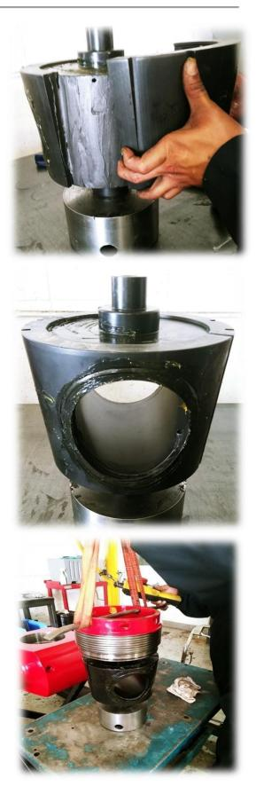
11. Use one of the three Giant Button Head Grease Fittings (#15) and the Flat Washer - ¾ (#14) to secure the Cap Body. Lightly tighten turning clockwise.
