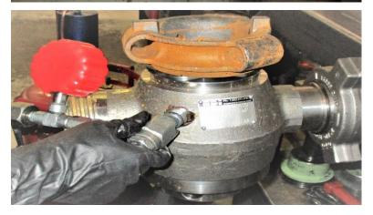
23. Remove the excess grease in the bore of the Plug Valve by pushing a clean rag through the bore.
