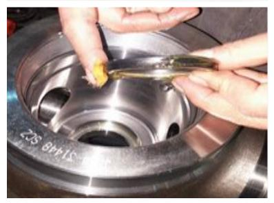
Pack the Cap Body (#15) with grease all around the open groove as shown. Apply grease into the seal pocket of the Cap Body and on Plug Seal (#10). Insert the Plug Seal into the Cap Body seal pocket - copper plate facing down.
