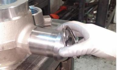
Slide the Wingnut (#18-2) next to the Snap Ring. Place the Segment Set (3) (#18.3) around the male end and pull the Wingnut over the Segments to hold them in place.
