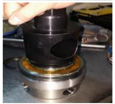
11. Turn the Cap/Plug Assembly upside down and secure it snugly with the ½" Hex Bolt (#1) and Washers (#2 & #3). Then apply a liberal amount of grease on the sealing surface of the Plug Body.
