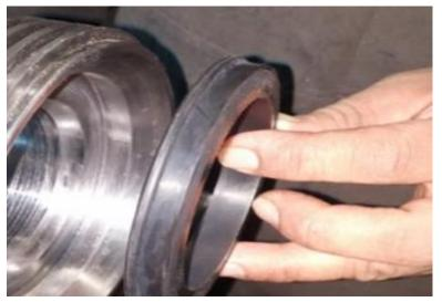
Mount the **Plug Valve Body** on a bench receiver.
