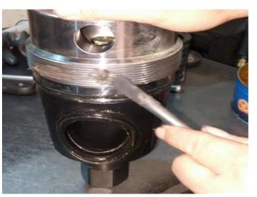
15. Apply a moderate amount of assembly grease on the internal wall of the Plug Valve Body, then slowly insert the Plug/Cap/Seat Carrier assembly into the Plug Valve Body while maintaining bore alignment with the bore of the Plug Valve Body.
