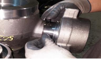
Insert the Union Seal (#9) into the inside groove at the female end of the Plug Valve Body.
