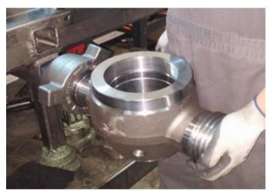
Insert and punch the Grooved Pins (#7) into the internal pin holes on both sides of the Plug Valve Body.
